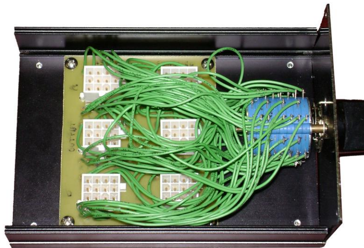
Figure 5.12 - AEVIT Controller Switch
