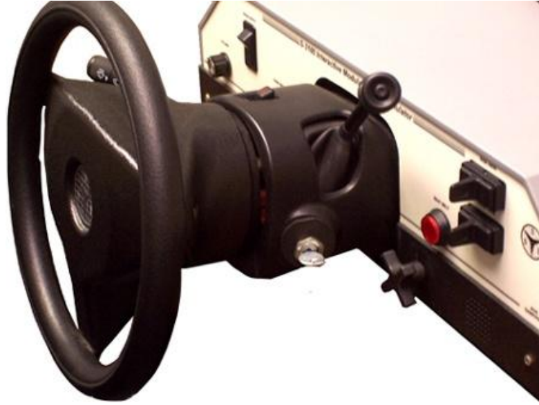
Figure 5.1 - SSI Modular Driving Simulator [37]
